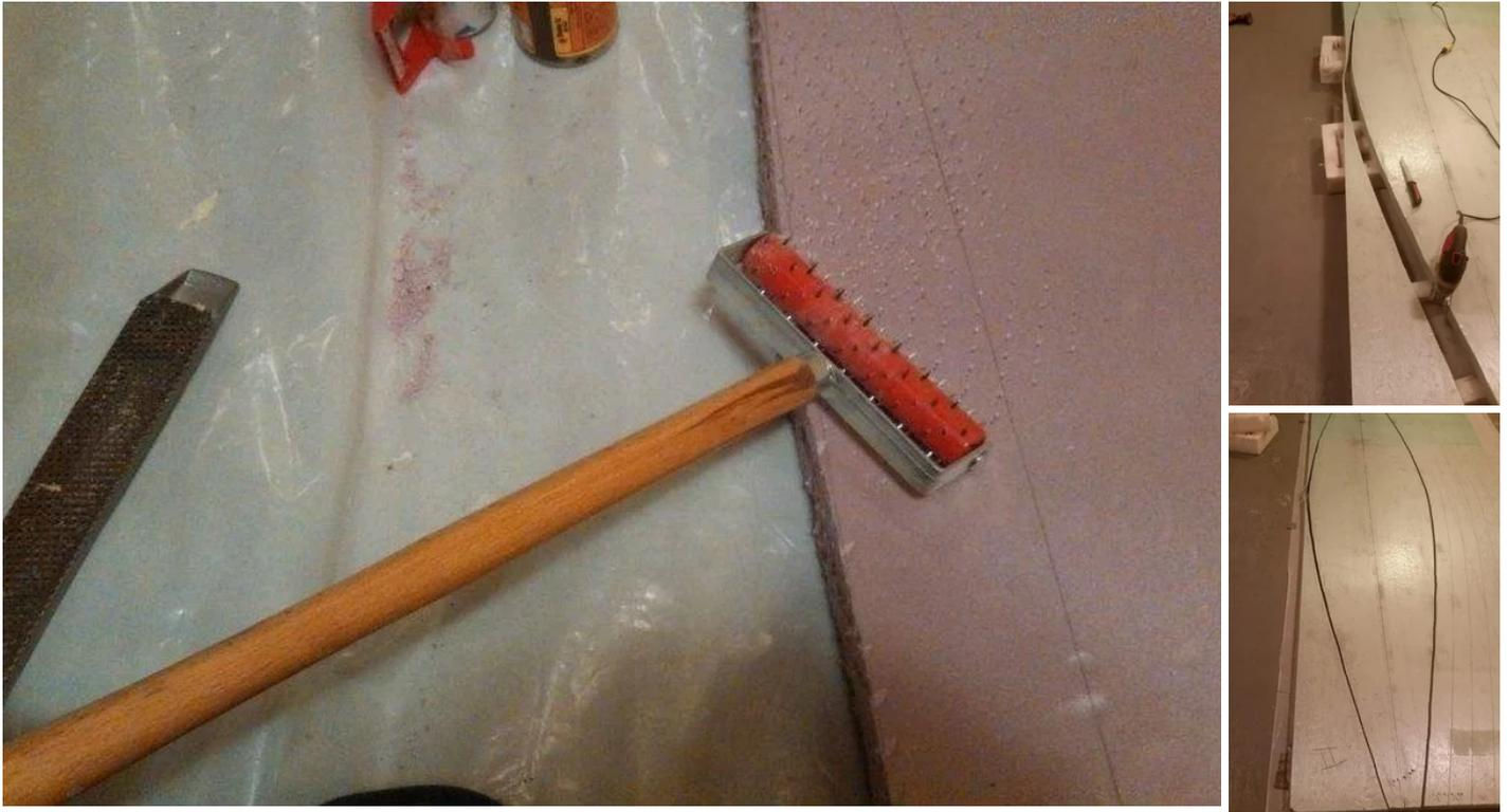
>Now take the wallpaper removal tool and score up the faces of each foam panel, each of the holes left by the spikes on the tool will allow glue to penetrate into the foam deeper. I prefer to think of the holes as becoming thousands of tiny nails that pin the glued joints together. Peeling of the fabric later on for modifications to the boats has proven this to be true.
