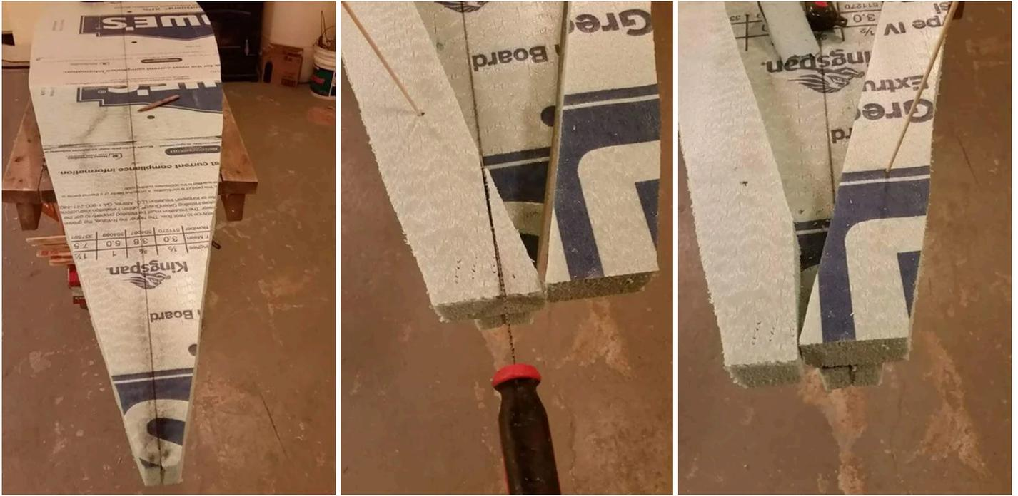
>copy the ends of the centerline on the bottom blank over to the other side of the foam.
